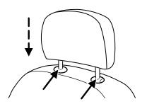
Properly adjust the head restraint so that the top of the head restraint is even with the top of your head and positioned as close as possible to the back of your head. For occupants of extremely tall stature, adjust the head restraint to its full up position.
